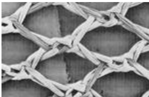
Gambar 5. Gambaran mikroskopik braided polypropylene mesh (5).
